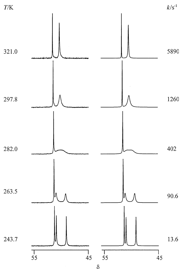
Fig. 2 Typical exchange 100.614 MHz ^{13}\text{C} - \{^1\text{H}\} NMR spectra of [\text{LuL}^1]^{3+} ( 0.025 \text{ mol dm}^{-3} ) in \text{CD}_3\text{CN} . Experimental temperatures and spectra appear on the left, and the best-fit calculated line shapes and corresponding k values appear to the right
